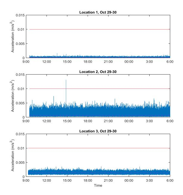
Figure 1: RMS particle accelerations at Location 1, 2 and 3 on October 29-30, 2017. The magenta dash line represents the mean baseline RMS particle acceleration calculated from October 5 to 16 at each location. The red line shows the 0.01 m/s<sup>2</sup> threshold of the RMS particle acceleration.
